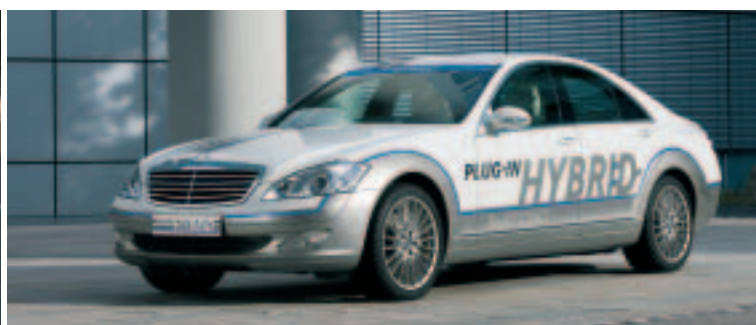
Vision S 500 Plug-in HYBRID 3,2 l/100 km, 74 g/km, 0–100 km/h 5,5 s
